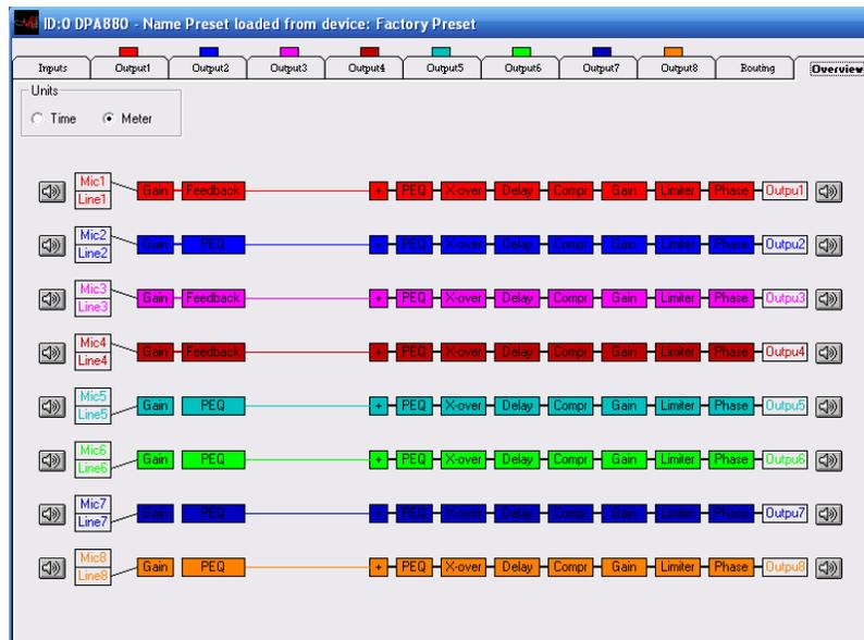
Within the Overview Page, can be checked the all channels inputs selection (between Microphone and Line), so as any of the available processes can be accessed double clicking on its name in the processes' block diagram.
