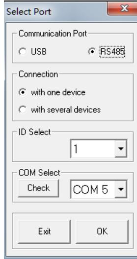
5. Click the "OK" button in below figure. If the DPA480P connects to the PC with RS485 successfully, then below interface will appear.
